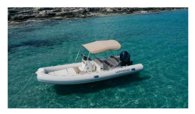
RIB with 6 meters in length with a 115 HP Yamaha outboard with a maximum capacity for 10 people. At the bow it has a large solarium, at the stern it has a double folding seat to have another solarium, bathing platforms with ladder and fresh water shower. On the bridge it has a gps-plotter, music with bluetooth.
